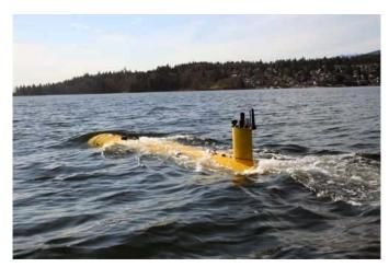
MARUM's new AUV, named SEAL, is rated to a depth of 5000 meters and has an endurance of 24 hours at a speed of 1.5m/s. This and a payload capability of 100kg provide the ability to conduct a wide variety of missions including seabed surveys or in the water column.
