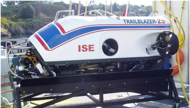
The ISE Trailblazer MCM ROV is a lightweight, highly manoeuvrable solution to mine detection, survey, recovery and disposal requirements. Developed by ISE specifically for MCM roles, the Trailblazer has successfully demonstrated its capabilities in Norway, Oman, Australia, the USA and Canada along with 4 other countries. Trailblazer is in current operational service with the Canadian Navy.
