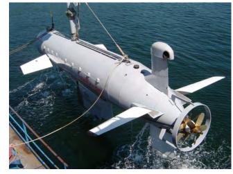
The Dorado vehicle is capable of towing a sonar towfish at speeds up to 12 knots and depths to 200 m. It is powered by a 315 kW marine diesel engine. Air is drawn through the mast and exhausted through the stabilzer above the contra-rotating propeller. The engine also provides power for the hydraulically operated control planes and the keel-mounted winch for the sonar towfish. The towfish is developed to follow the seabed at low altitudes and is fitted with a multibeam sidescan sonar.
