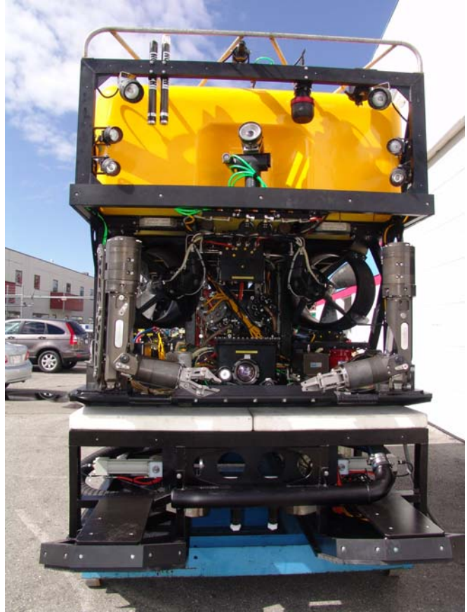
Figure 21 Hysub 150 with Jetting Skid - Side View
