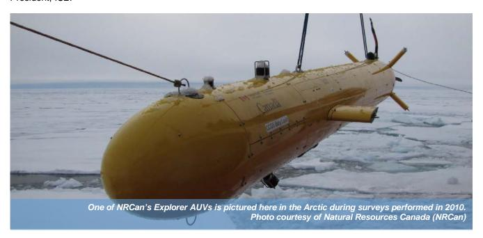
This *Explorer* AUV will be equipped with an EdgeTech 2205 sonar which incorporates side scan, sub bottom and bathymetric capabilities in one compact package. *Explorer's* modular design and unmatched dry payload volume provides opportunity for the AUV with room to grow, allowing UTAS researchers to adapt to the surprises that are inevitable when exploring never before seen areas of the ocean floor. New sensors and payloads can be integrated quickly and easily to adapt to new discoveries.
